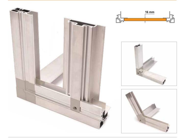
The Pileo system permits the production of frames with 16 mm thick panels. This system is unusual in that it allows one to cut panels produced in-house with a simple circular saw. Simple sheets are cut into panels for frames, such as door panels, with the PILE0000-2 profile . The PLBP-00000 "panel block", instead, is used to fasten the fixed panels in a secure and efficient manner (without need for further framing). This eliminates the need for expensive sheet processing centres.
