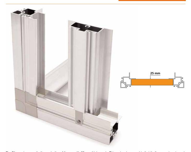
The Pileo system permits the production of frames with 25 mm thick panels. This system is unusual in that it allows one to cut panels produced in-house with a simple circular saw. Simple sheets are cut into panels for frames, such as door panels, with the PILE0000-1 profile . The PLBP-00000 "panel block", instead, is used to fasten the fixed panels in a secure and efficient manner (without need for further framing). This eliminates the need for expensive sheet processing centres.
