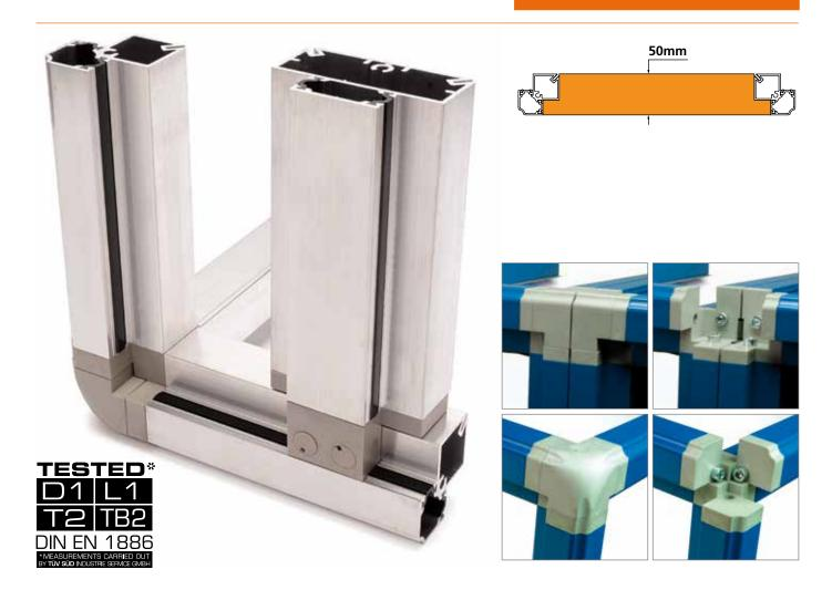
The Thor system is based on the screw tightening between the corner and the profile.
