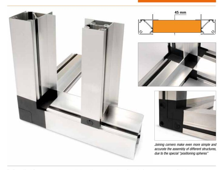
The Thermal Break Stopper system reduces assembly time and increases the sturdiness of large-size frames: just insert the profile in the slots on the corners and secure in place with M6 screws. The structure of the module is completed by a nylon cover and cap, which ensure perfect closure. The two apecial "positioning spheres" on the joining corners also allow an obvious simplification in the process of joining different cubes.
