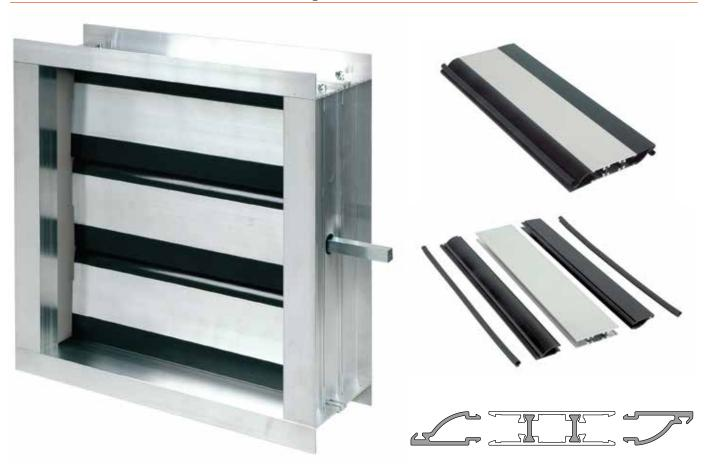
Built with the same components of the standard frame, it introduces a blade profile with thermal break to improve the total power efficiency. Blade PS100TT-00 enables a reduction of the thermal exchange on 90% of the surface, maintaining the same assembly system for the damper. This profile, which has the same sizes as the PS10000000 blade profile, includes a thermal break aluminium profile assembled with two PA 6.6 profiles.
